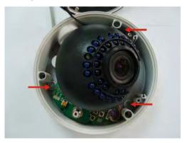
4. Arrows point to the 3 holes for ceiling mount screws
